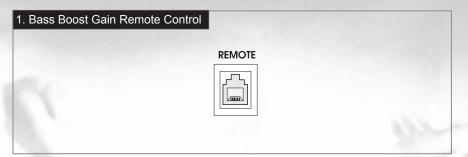
This plug connects the amplifier and the remote bass knob using the supplied cable.
